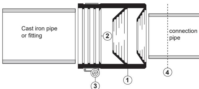
1. Put completely delivered SIMA-CON (1) onto tube end or fitting up to distance ring (2). Fix with tensioning strap (3) (cross slot, SW 7, rec. torque 2 Nm).
