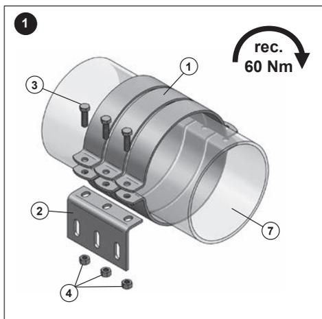
1.) Fix suitable MEFA fixpoint clamp (1) on pipe (7). Mount side part (2) under straps of pipe clamp. Attract screws (3) and nuts (4) with torque of 60 Nm.
