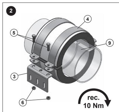
2.) Mount Side part (3) of recommended Fixpoint bracket HV under straps of outer split ring (4). Attract screws (5) and nuts (6) with torque of 10 Nm.
