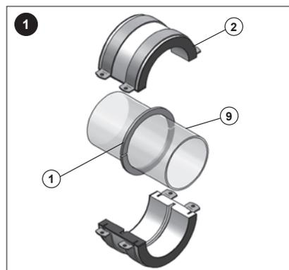
1.) Weld inner split rings (1) of insulated fixpoint to steel pipe (9).
