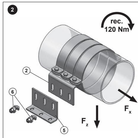
2.) Install stilt (5) using T-lock (6) on side panel (2). Adjust desired height and attract with torque of 120 Nm. Fix entire construction on any suitable substructure (e.g. C-profile rail, CENTUM, steel beam).
