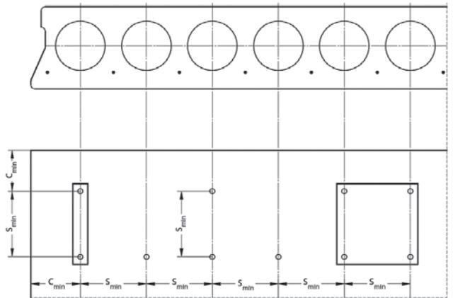
Minimum edge distance  $c_{min} \geq 150$  mm
