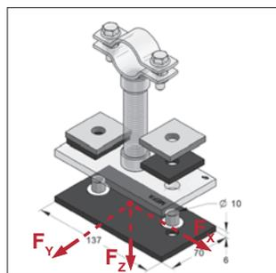
Sound-decoupling set for the clamped fixpoint
