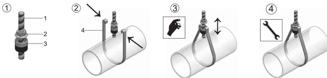
1. Mount threaded rod (1) into dowel/anchor. Fix flange nut (2) onto threaded rod (1). Allocation as per margined table. Push cup nut (3) from down across threaded rod (1).
