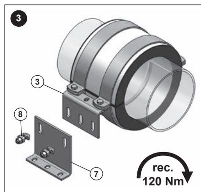
3.) Install stilt (7) using T-lock (8) on side panel (3). Adjust desired height and attract with torque of 120 Nm. Fix entire construction on any suitable substructure (e.g. C-profile rail, CENTUM, steel beam).
