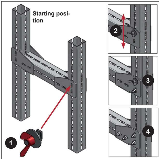
2. **Align:** To align the profile, loosen the CENTUM® FixBOB and tighten again (hand-tight only) after reaching desired position/location.
